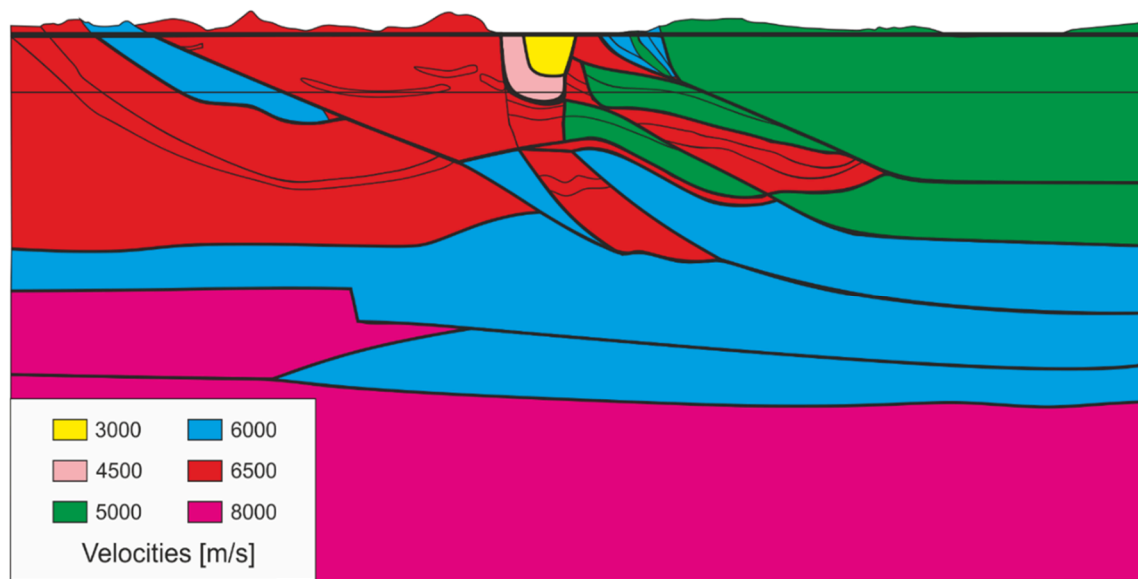
Figure S3: Simplified P-wave velocity model of the reprocessed seismic section for depth conversion. Generated on a first conceptional interpretation of time-migrated stack. Modified from Galler et al.
